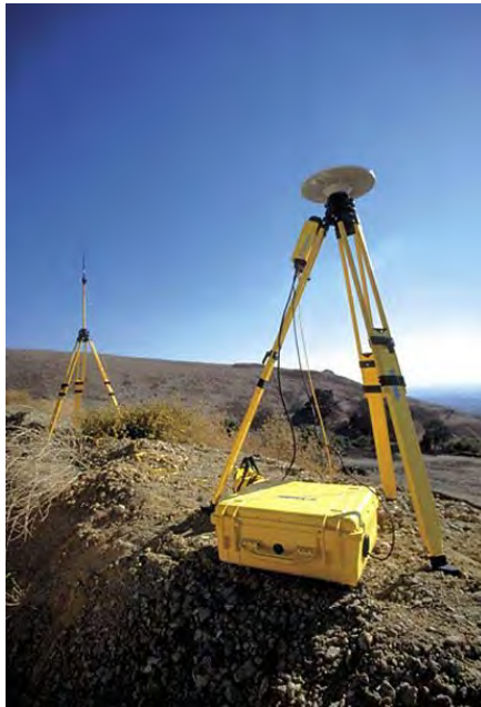
Reference (Base) Station
