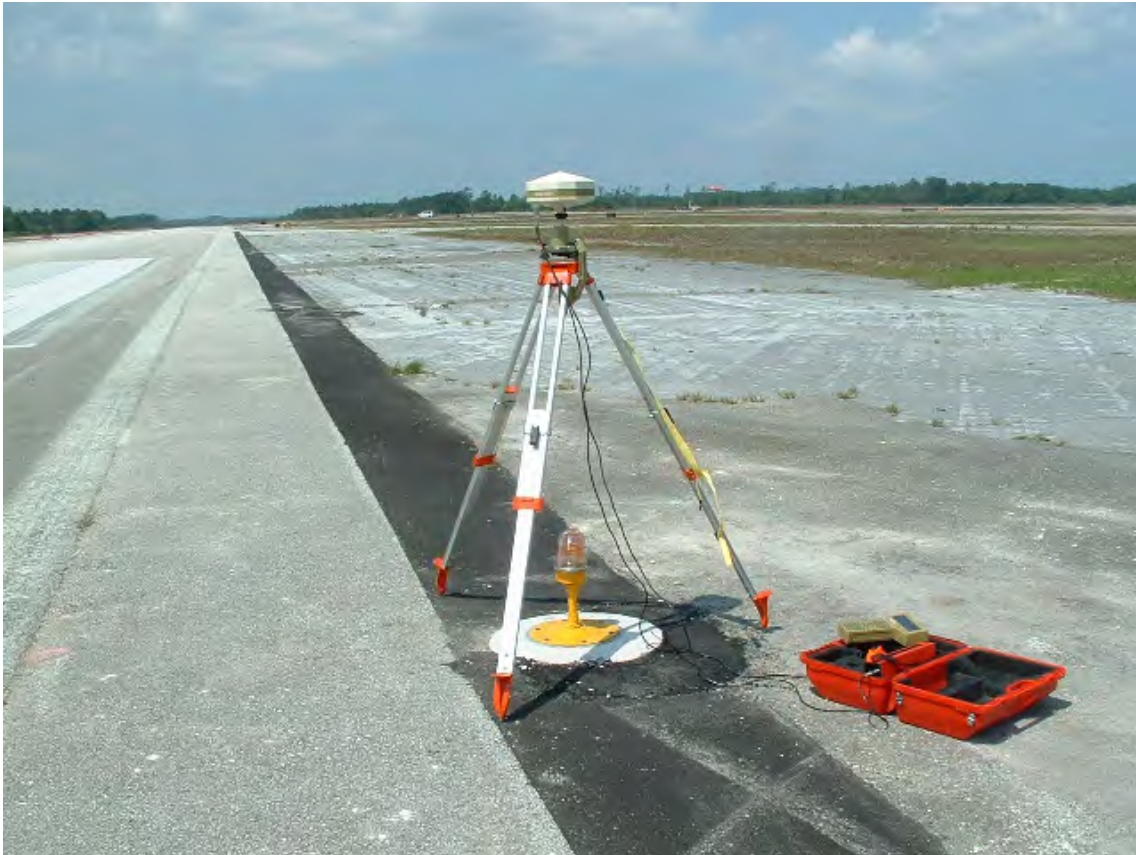
Figure 2-3. Airfield NAVAID positioning using Fast-Static GPS methods
