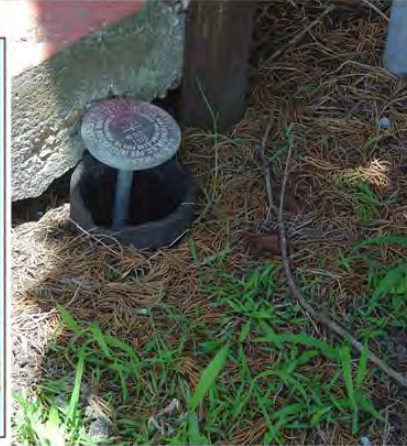
Figure 5-14. Estimated subsidence (in centimeters) in the New Orleans to Venice region. Photos depict relative ground subsidence of benchmarks attached to deep driven rods.
